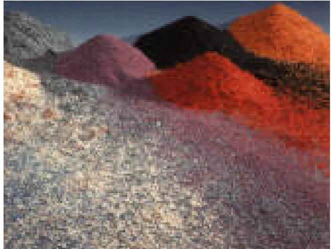
The concept is simple. It is a combination of floor flakes and floor resin. A new product is "born". The floor resin plays a leading role in the quality of the flooring system. The color flakes provide the additional decorative effect.
